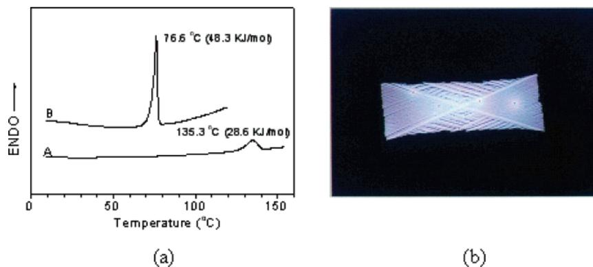
**Figure 3.** (a) DSC curves recorded during the first heating scan of (A) **1** and (B) **2**. (b) Representative optical polarized micrograph (100 $\times$ ) of the texture exhibited by **2** at the transition from the isotropic state at 76  $^{\circ}$ C.
