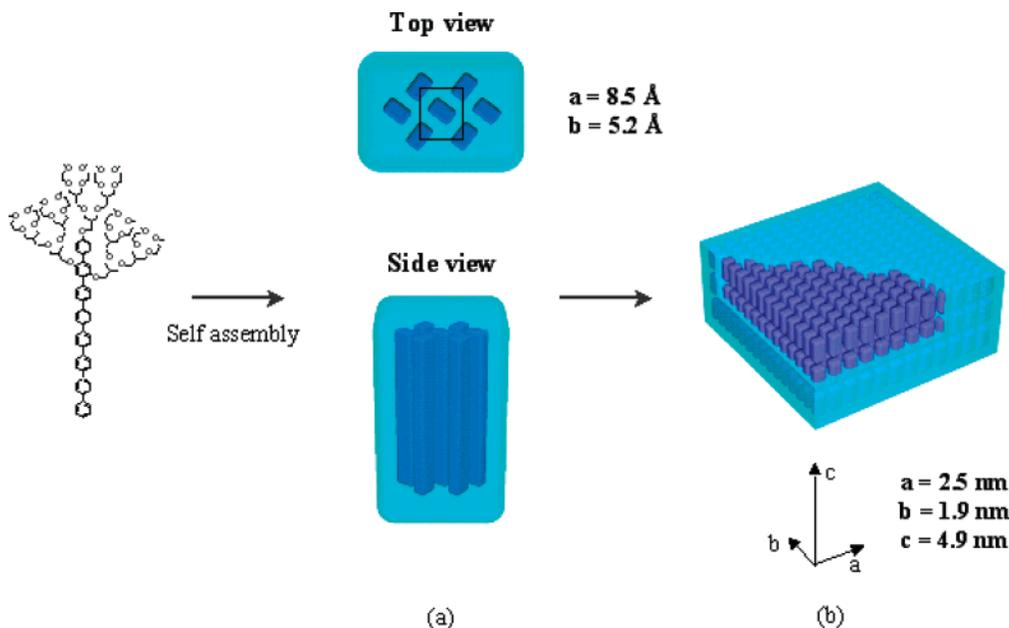
**Figure 6.** Schematic representation of (a) the self-assembly of **2** into a discrete bundle with the herringbone packing of the octa-*p*-phenylene rods and (b) the subsequent crystallization into a primitive orthorhombic superlattice.
