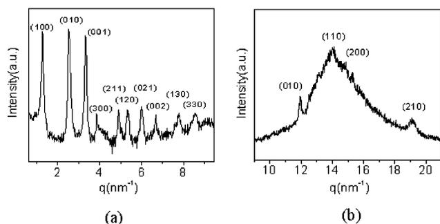
**Figure 4.** (a) Small-angle X-ray diffraction pattern of **2** measured at 25  $^{\circ}$ C. (b) Wide-angle X-ray diffraction pattern of **2** measured at 25  $^{\circ}$ C.
